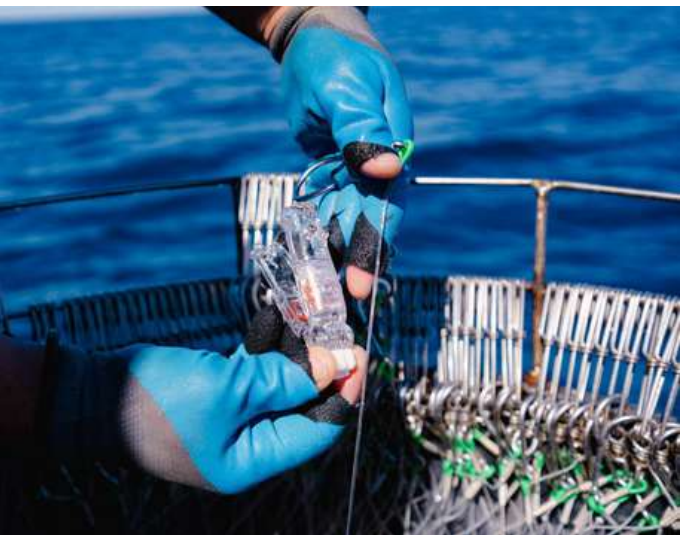
Deployment of hookpod devices for releasing hooks of floating longline gear underwater (Author: A. Gugić)
