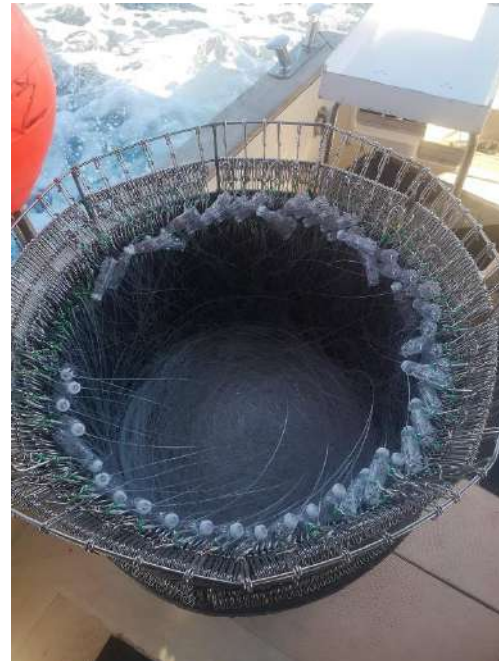
Figure 3 Testing devices for releasing drifting longline hooks under sea surface (hookpods)
