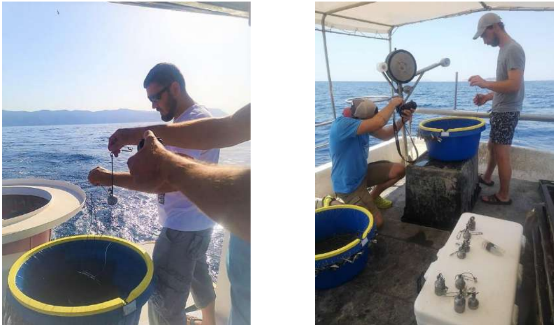
Figure 2 Testing additional weighting (weights) on demersal longlines
